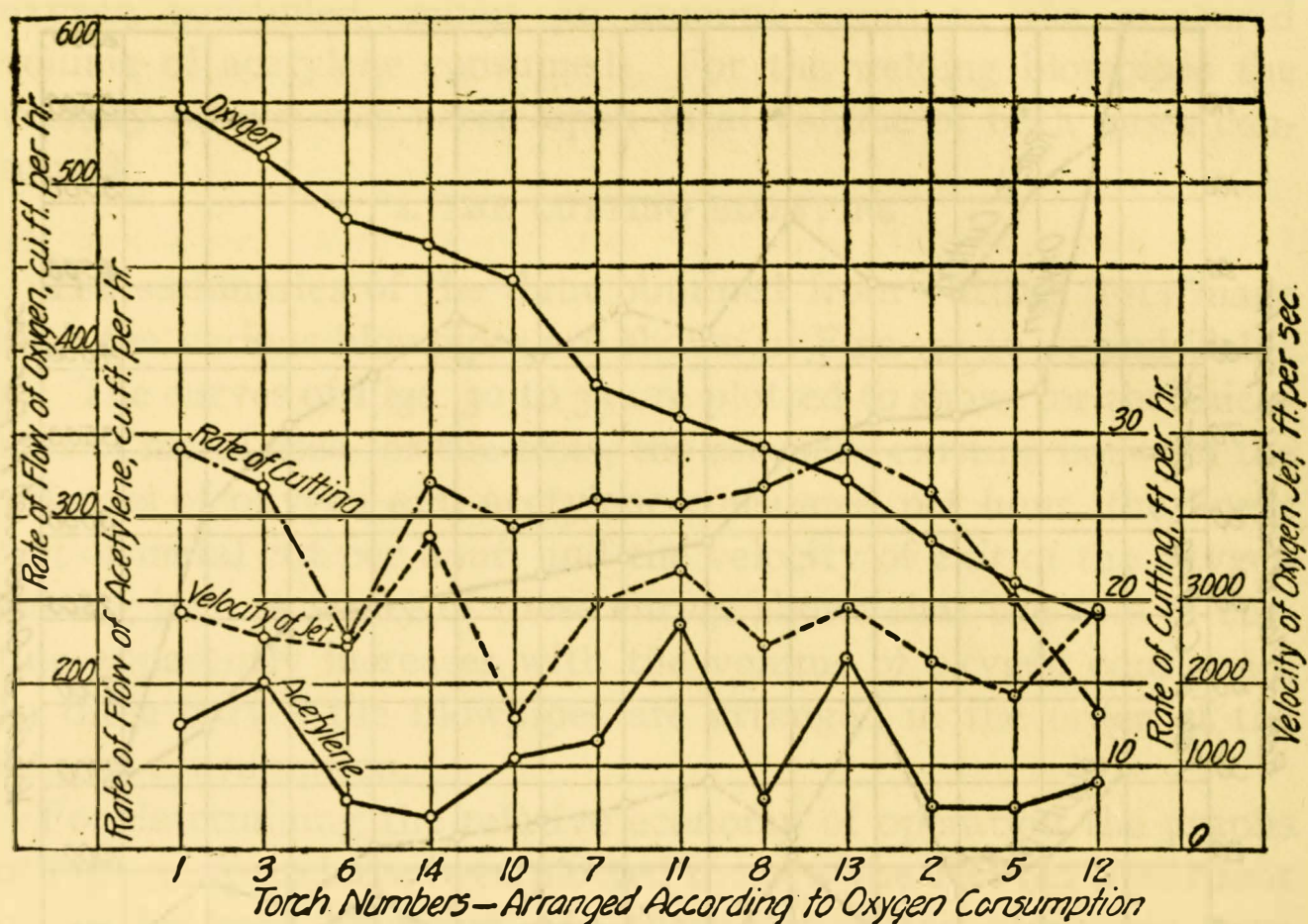
FIG. 34.—Relation of rate of flow and velocity of exit of oxygen to rate of cutting 6-inch metal
