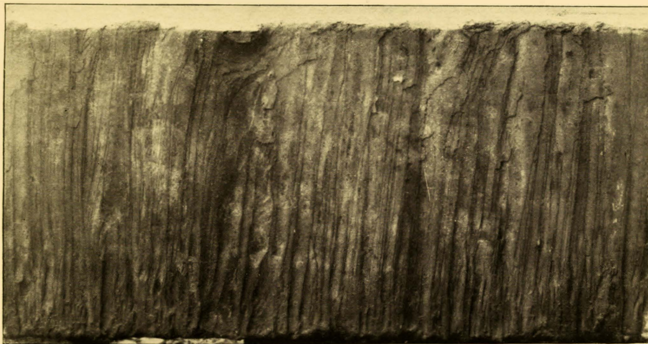
FIG. 46B.— Oxyhydrogen cut on 10-inch steel showing relative smoothness of cut
