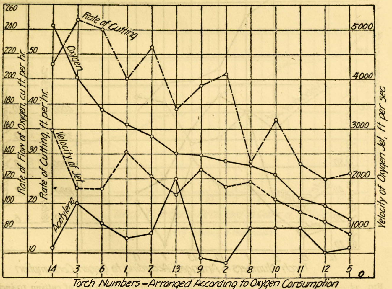
FIG. 33.—Relation of rate of flow and velocity of exit of oxygen to rate of cutting 2-inch metal
