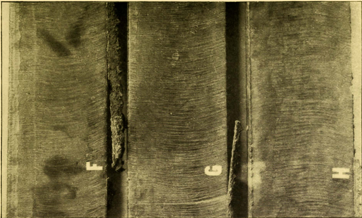
FIG. 43.—Oxyacetylene cuts on 6-inch steel
