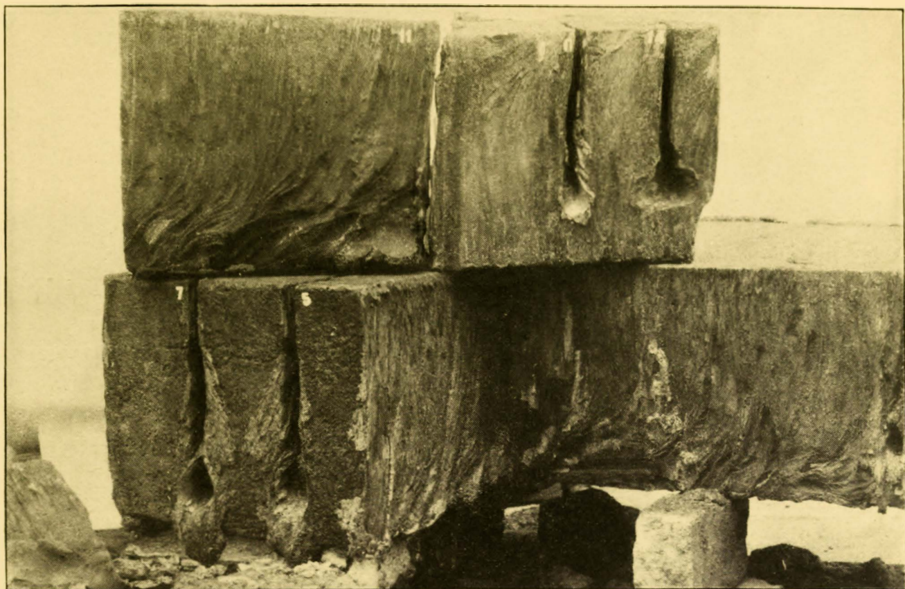
FIG. 46A.— Oxyacetylene cuts on 10-inch steel showing failure to complete cut
